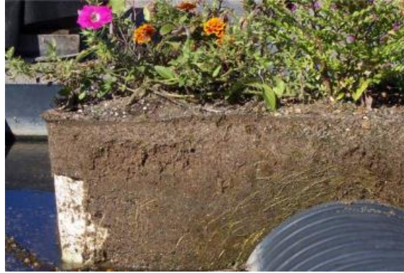
Figure V - EPIC sand capillary zone above saturated zone
